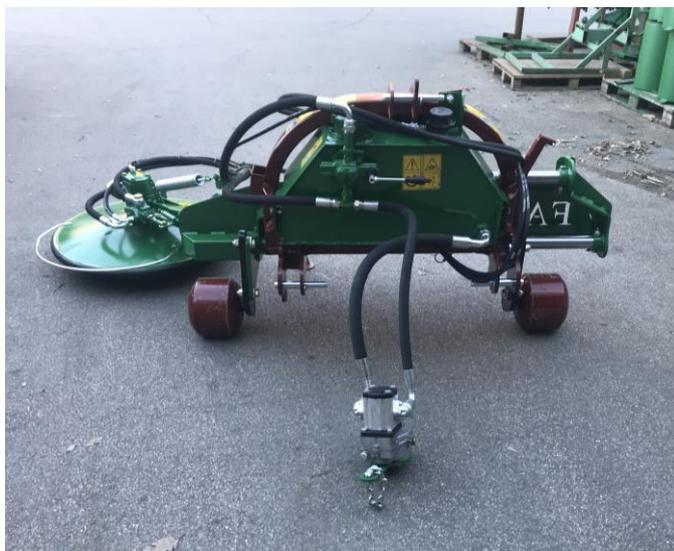
**Independent hydraulic inter-row disk**, directly applicable to the tractor by the third point linkage. It is powered by the power take off and linked to the tractor hydraulic clutches. It is endowed with: oil tank, pump, distributor, hydraulic clutches for the coupling and uncoupling, multiplier, kit for lateral displacement. **Kit hydraulic sensor on demand.**
